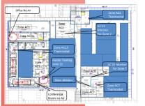
The integrated energy and equipment monitoring also produced notifications of equipment failures continuously in real time. Examples of faults detected in this building, often within minutes, include failure of one stage of cooling, stuck economizers, broken fan belt, breaker left off after preventive maintenance, etc.
